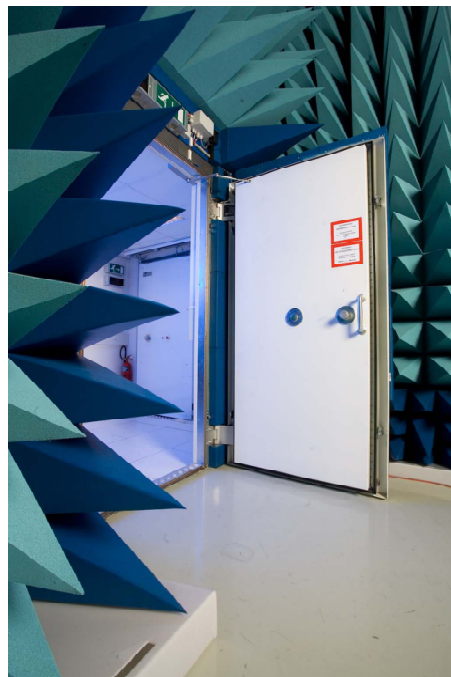
Low threshold for ease of move in and out of the chamber
