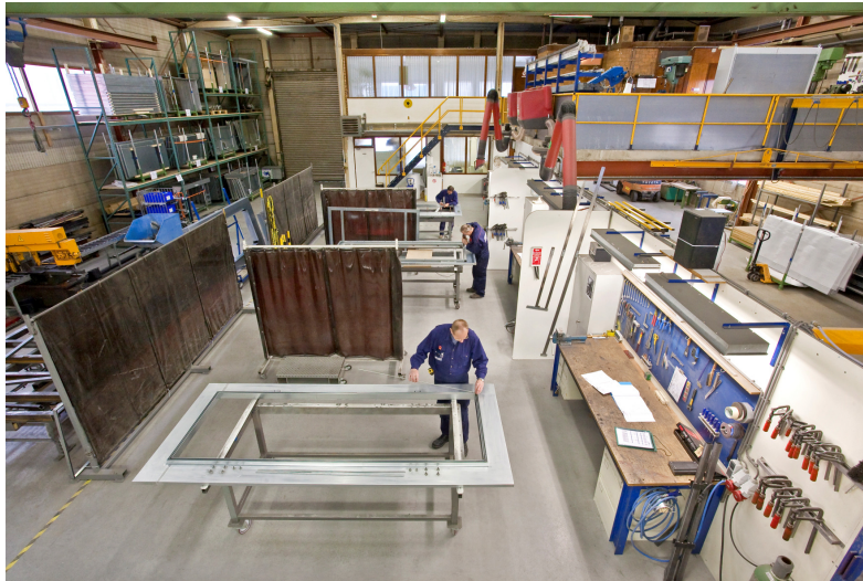
Assembly of shielded doors
